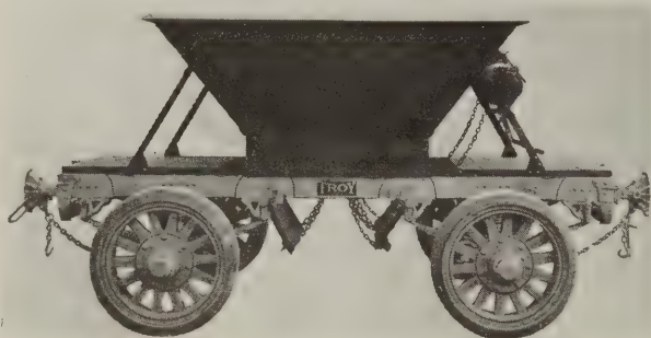
A DUMP TRAILER WITH A CAPACITY OF THREE CUBIC YARDS.
